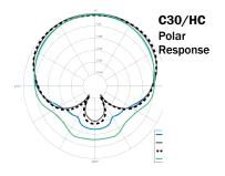
uniform over its operating frequency range; the frequency response at 90 degrees off-axis is very close to the on-axis response. Such uniform polar response results in less phase problems on the sides of the microphone and there are fewer phase cancellations when using multiple microphones placed close together. This new microphone technology also provides more rejection of unwanted sounds from the rear of the microphone and more gain before feedback in live sound applications.
